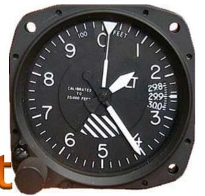
**Indicated altitude:** the approximate height of the aircraft above mean sea level [MSL], calculated in accordance with the ISA.
