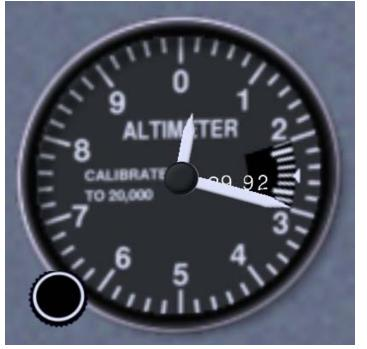
True altitude: the actual height of an object above MSL. (Objects on aeronautical charts are in true altitude.)
